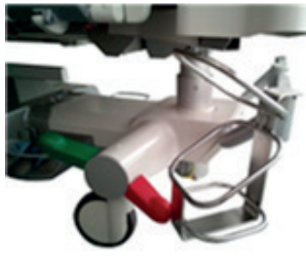
Fig. Oxygen Bottle Holder B – incorrect fitment
