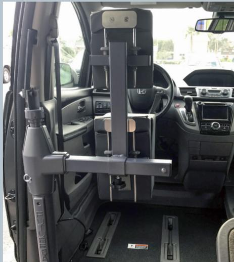
eFutureSafe folded out; suitable for almost all common wheelchair types
