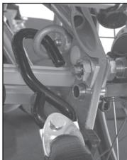
In rear: Mount an "eye-bolt" in one of the holes in the wheel frame bracket. Hook on a hook/ carabiner in the "eye-bolt" The angle of the straps should be 0-45° Item number for 1 pair of eye bolts with bushing: 21074.
