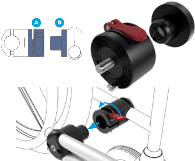
"M3D Base Coupler" Coupler with a quick release mechanism. Connection guided by a magnet. Adds a 38 mm offset (1 1/2"). complete 11.1550 A inner part 11.1551 B outer part 11.1552
