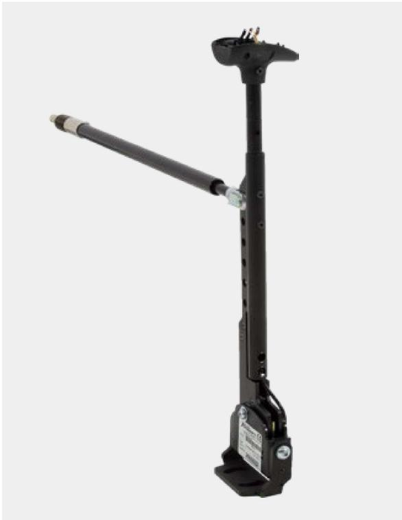
The Carospeed Menox moves the control of acceleration and brake from feet operated pedals to one hand operated lever. Pull the lever to accelerate and push to brake. Menox is designed to make each control ergonomic, conforming to a person's natural hand-wrist-arm motion.
