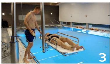
Position the client with the stretcher or wheelchair above the water. When the client is in the correct position, lower the stretcher or wheelchair.
