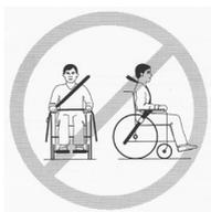
MAKE SURE THAT ARMRESTS, WHEELS AND OTHER COMPONENTS DO NOT PREVENT BODY CONTACT. THERE MUST BE FULL BODY CONTACT WITH THE 3-POINT STRAP.
