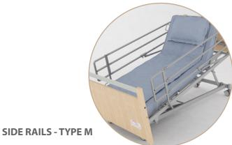
The Metal Side Rails system is equipped with a 3/4th length side rails of a bed's length and protects a patient up to 385 mm of height. Side rails locking system in upper position is operated automatically. Side rails dropping system is not available for the patient and can be only operated by personnel. Metal Side Rails System can be easy and fast operated and doesn't require any additional space. Metal side rails are manufactured according to current norm EN-60601-2-52.
