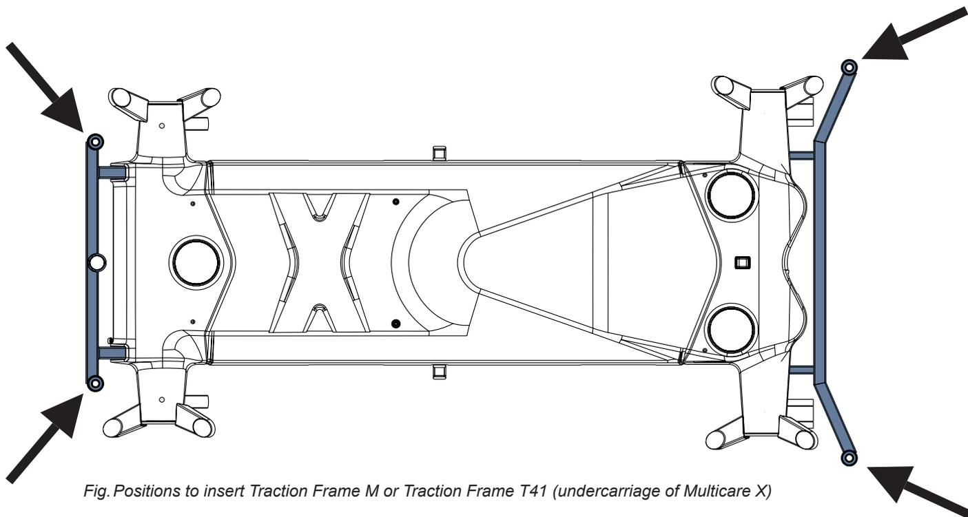
Fig. Positions to insert Traction Frame M or Traction Frame T41 (undercarriage of Multicare X)
