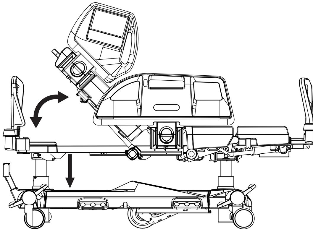
In Mobilisation Position bed is descending to the lowest Bed Height and Backrest reaches the maximum angle.
