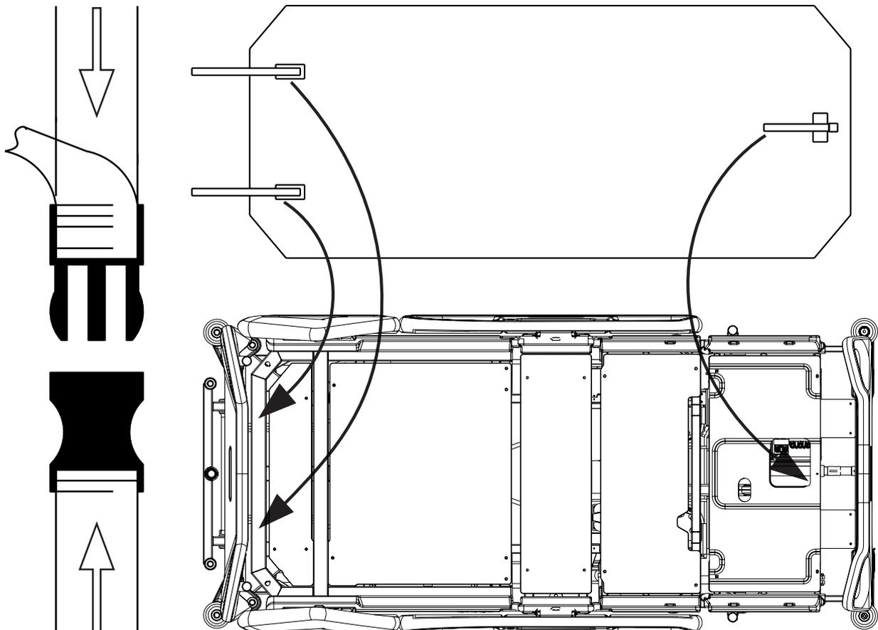
Fig. Fixation of the mattress with straps on the mattress support platform of Multicare X bed
