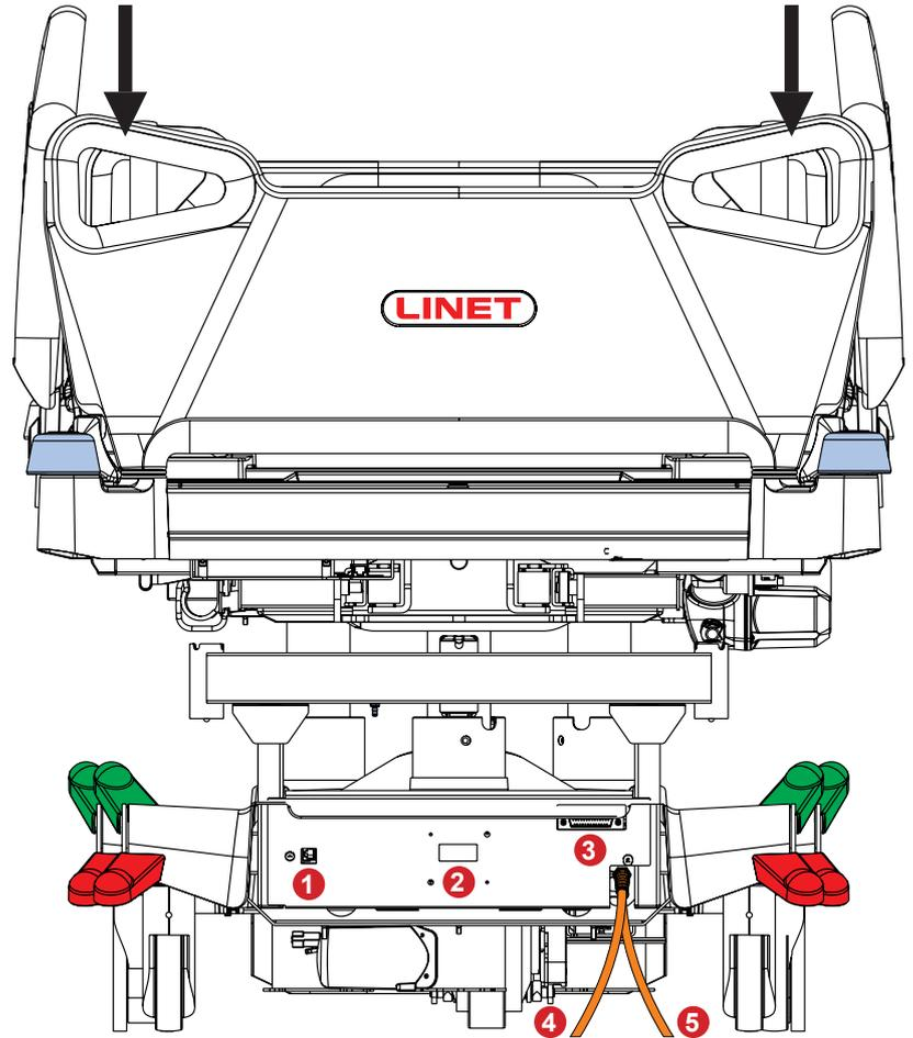
1. LAN connector (to connect the medical bed to a LAN data network)
