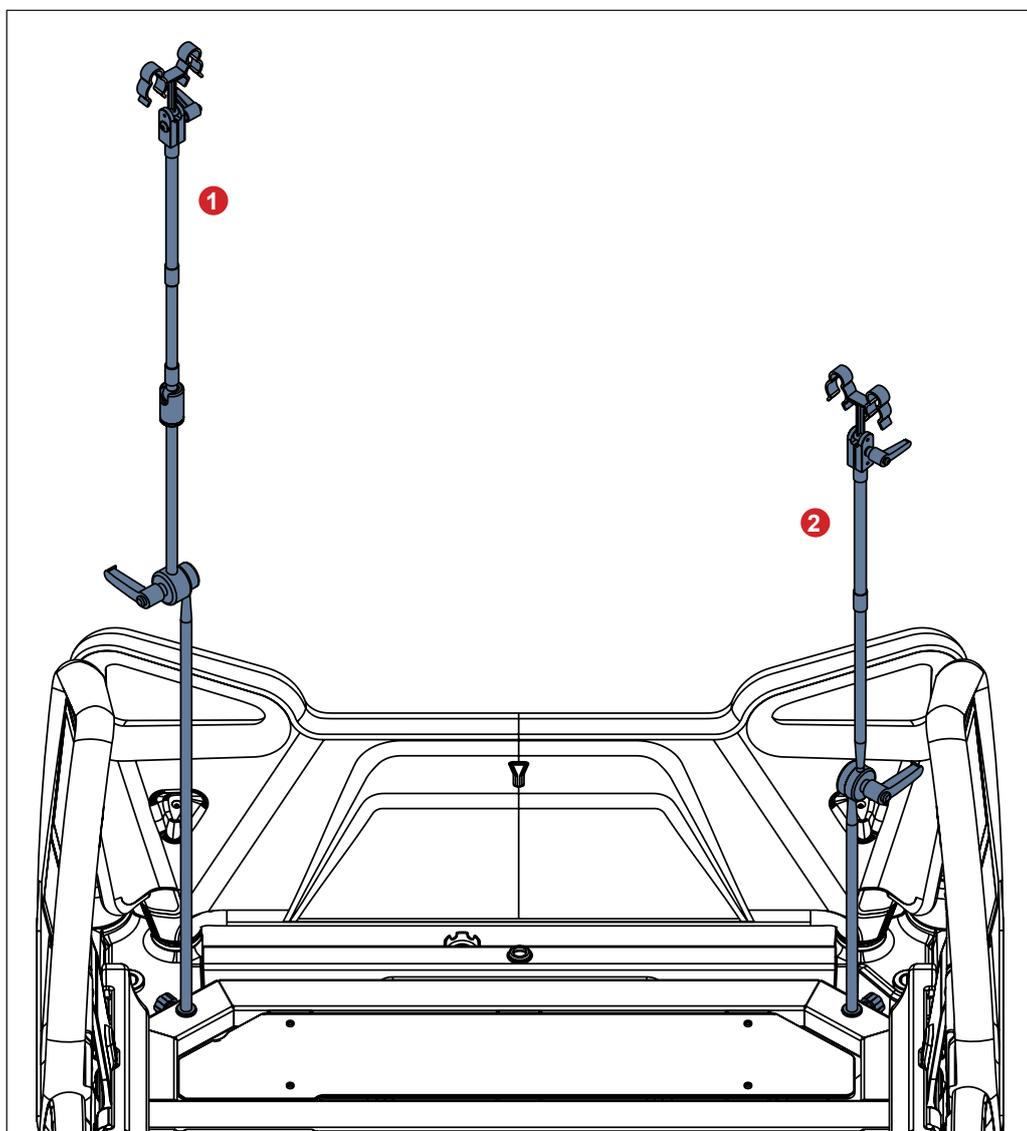
Fig. Ventilation Circuit Holders placed on the Backrest
