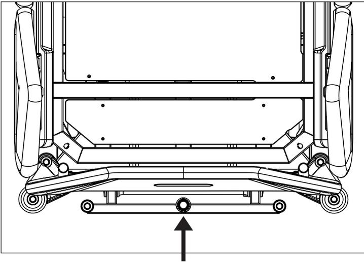
Fig. Places for lifting pole (sleeve fitting on accessory adapter)
