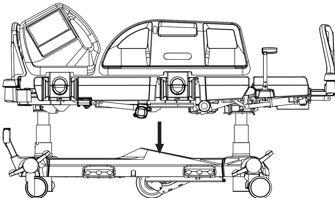
In CPR Position bed reaches flat Mattress support platform.
