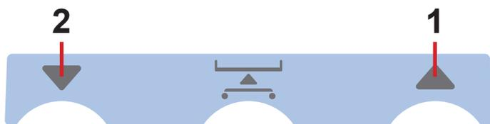
Fig. Bed Height Pedals (Bed Height Foot Control)
