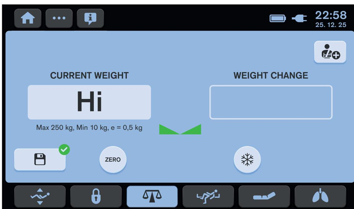
Fig. First degree of the bed overload (displayed Hi)
