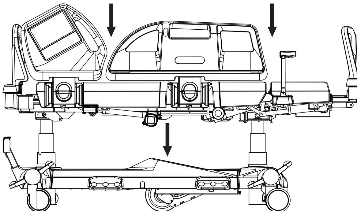
In Low Flat Position the mattress support platform is firstly adjusted to flat position without any lateral tilt and then lowered to the minimum height.
