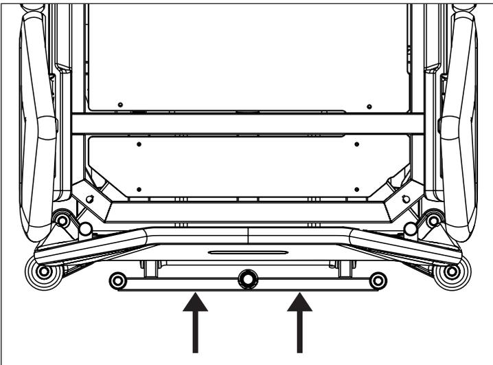
Fig. Places for Horizontal Oxygen Bottle Holder
