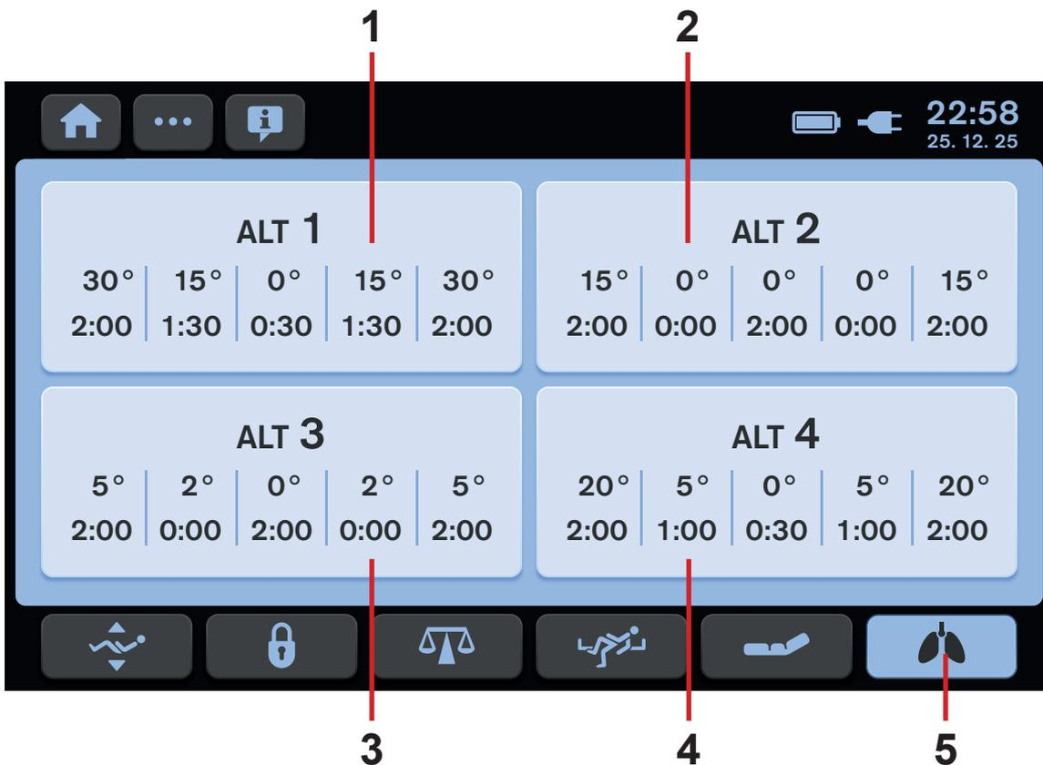
Fig. Initial ALT screen with 4 preset ALT programs
