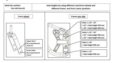
With wheel combination 22" + 6" the seat height 440 and 475 mm is possible.
